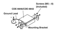
• Secure the ground lead of the unit to a clean metal spot using a screw (\*) already attached to the vehicle's chassis.
